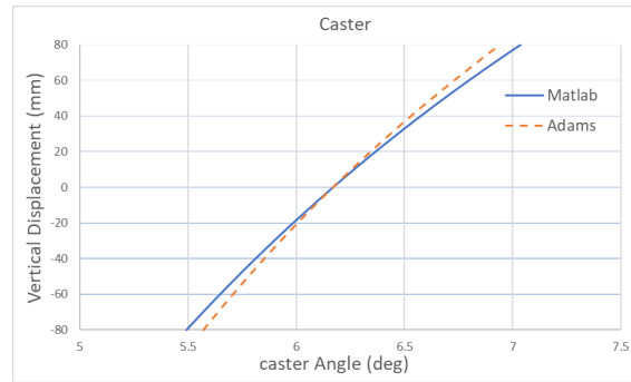
Figure 7 Caster angle vs. wheel travel
